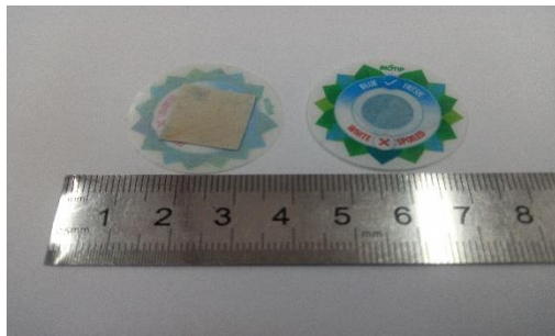
Fig. no. 1: Freshness Indicator Sensor(PP printed film +sensor), R-3868.
